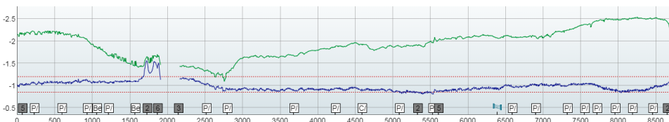
Figure 1C: CIP Survey Graph (Pipe-to-soil, V_{CSE} vs. Length [ft])– Target and Foreign ICCP Systems Synchronously Interrupting.
