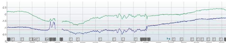
Figure 1A: CIP Survey Graph (Pipe-to-soil, V_{CSE} vs. Length [ft]) – Target Line ICCP Systems Interrupting.
