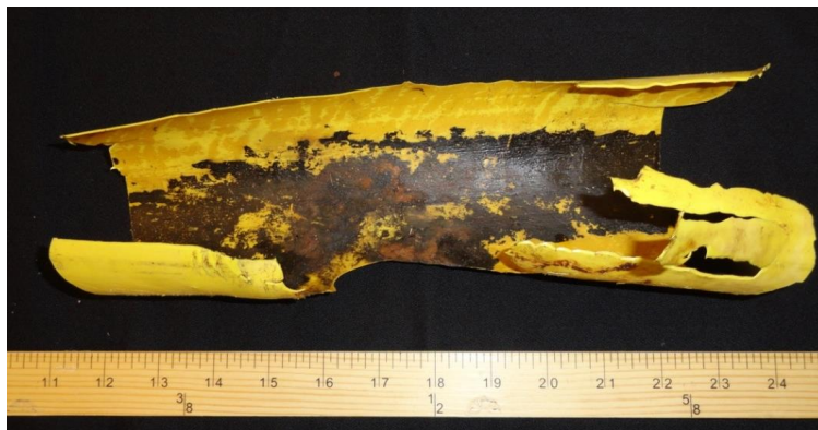
Figure 14: Photograph of the plastic extruded coating separated from the pipe.
